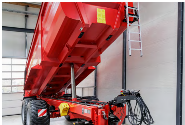
New and innovatively designed body beams.
