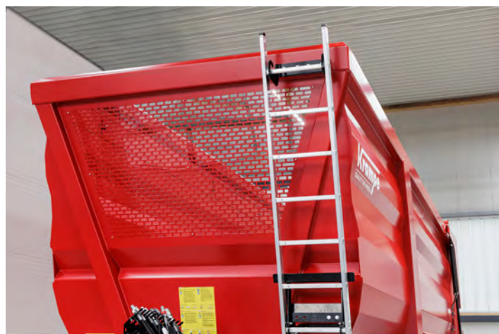
Angled front wall with large inspection window – the load is always in view.
