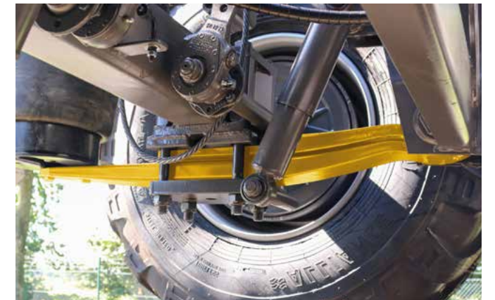
As standard with two-bladed pull rods and pneumatic suspension
