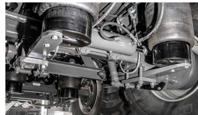
BPW caster steering axles: Design with pressure axle disc for smooth driving behaviour. The steering axle must hydraulically be locked when driving on roads.
