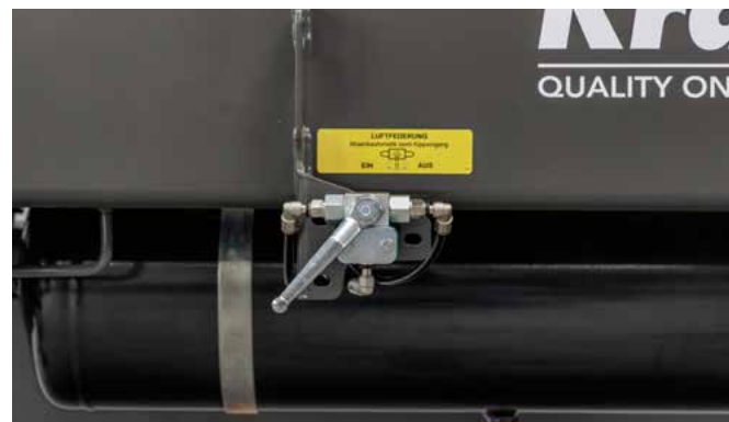
The pneumatic suspension is equipped with a reverse tap as standard. This can prevent from lowering of the running gear during tipping.
