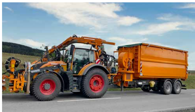
Volume container with blow-in opening for the transport of grass cutting which are mown from the roadside verge and the vacuumed.
