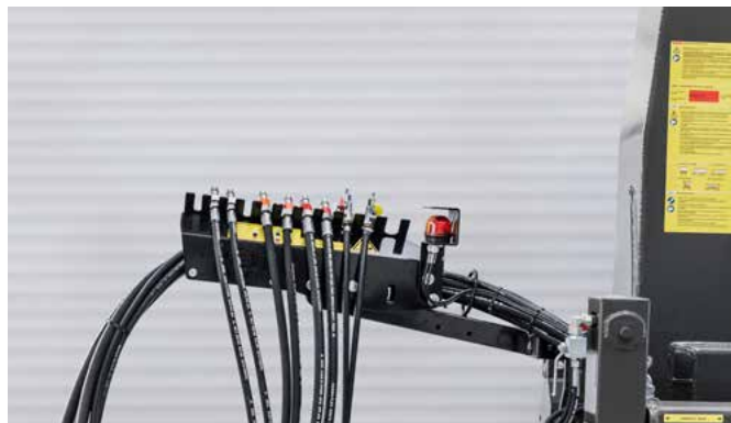
The THL 25 L uses the tractor hydraulic system. Container weights of up to 25 t can be picked up and unloaded. An auxiliary tipping cylinder is mounted as standard.
