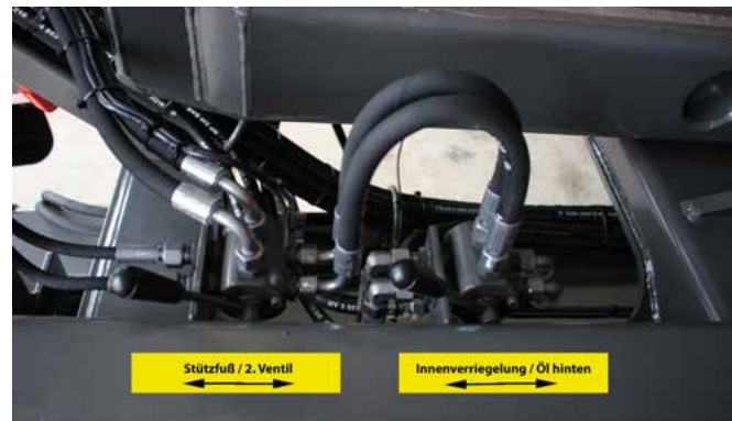
Two hydraulic functions can be operated with one control unit by means of the 6/2 way valve.
