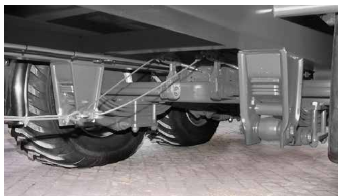
Export version: The construction height is very low for the version with parabolic springs and suspended axles. A hydraulic rear axle support discharges the traction head during pick-up procedure.
