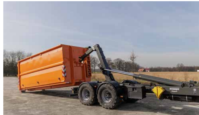
By foregoing an additional subframe, the pick-up angle is reduced and the pick-up performance increases.
