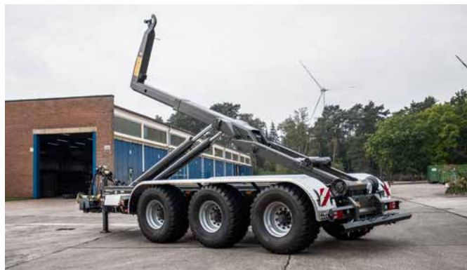
The THL 25 L is designed for container lengths of 6.5 m up to 7.0 m as standard.
