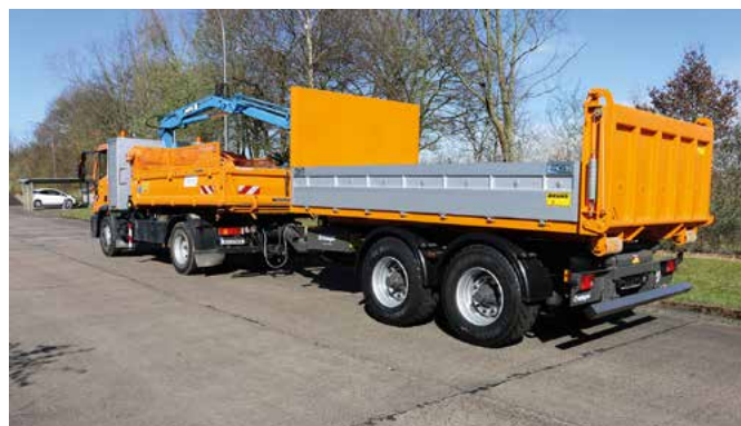
Municipal container with laterally foldable alu racks and traversable pendulum rear tailgate.
