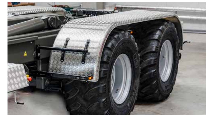
Alu mudguards for wide tyres and steering axles.
