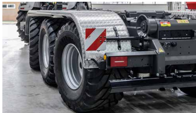
Our Tridem hooklift trailers are equipped with a caster steering axle as standard, but we recommend a forced steering.
