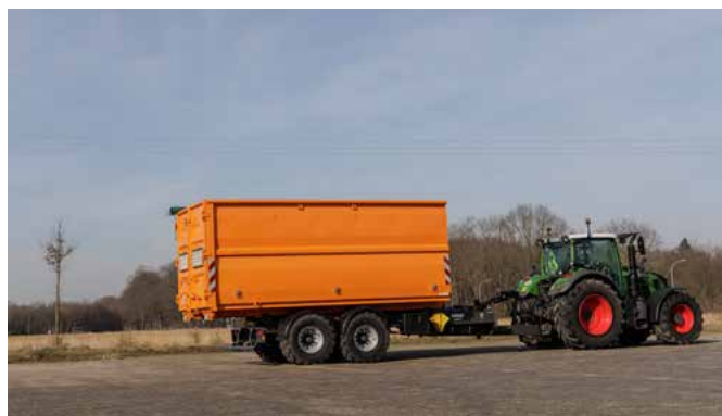
Container inside lengths of 6.25 meters or 6.75 meters resp. with a fold-out underride guard are possible.
