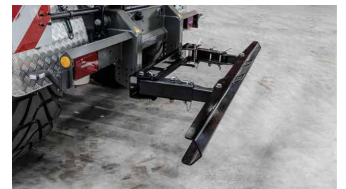
The foldable underride guard (effective stroke 50 cm) also allows the transport of extra-long containers.
