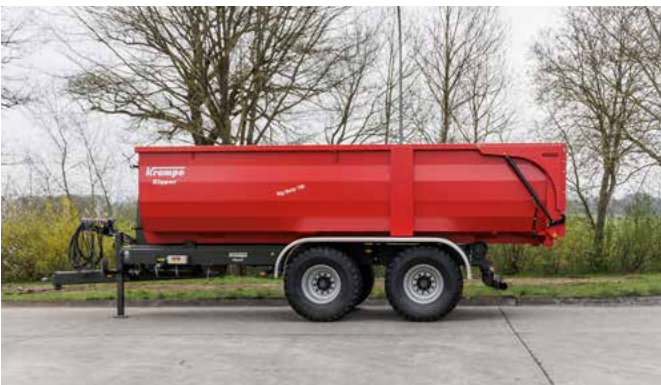
The THL 21 L with pneumatic running gear as standard can be supplied on request with a steering axle and a wheelbase of 1.81 m for a permissible GVWR of 24 tons at 40 km/h. For this model, a lot of further optional extras are available.
