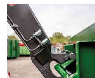
The hook seat has cleanly rounded contours. A height-adjustable hook is available as well as an oil connection at hook hoist.
