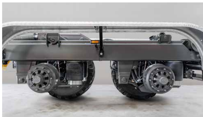
The pneumatic running gear is equipped with two-bladed pull rods and air bellows with a diameter of 360 mm. This combination ensures an extremely good and stable driving behaviour.
