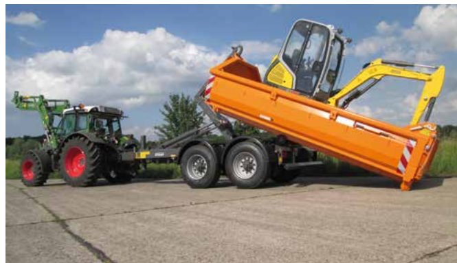
Container for the transport of construction machines with integrated lashing eyes and rear tailgate with double folding door.
