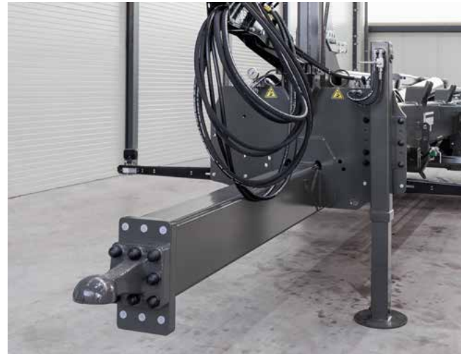
The classic towing device with hydraulic support foot.
