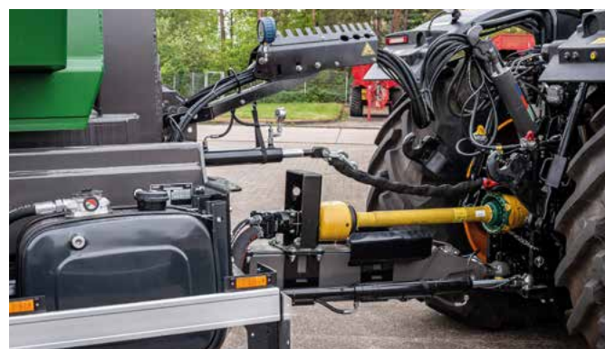
For all roll-off tippers up to 25 t lifting capacity, the hydraulic system (200 bar) of the tractor is sufficient. An independent oil supply with p.t.o. shaft is available upon request. A wireless remote control is included in the scope of delivery.
