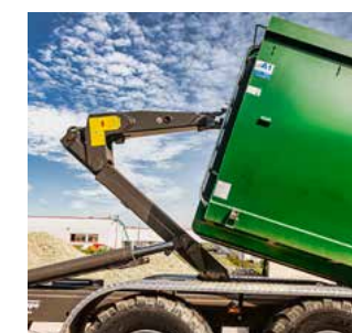
Optional articulated push arm version, for an especially flat lifting angle.
