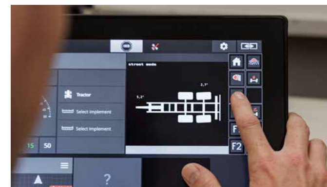
By means of an ISOBUS control, we have implemented the operation via the terminal of the traction vehicle for forced steering.
