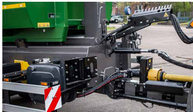
The THL 30 L is equipped ex-works with an independent oil supply and a wireless remote control. Containers with an own weight of 30 t can therefore be safely picked-up and tipped.
