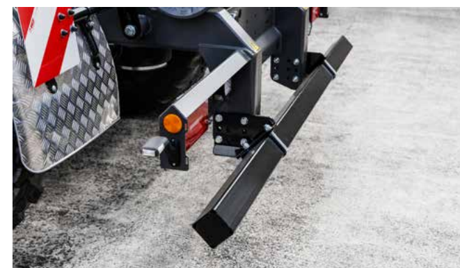
Rigid underride guard with COC approval for the 40 km/h version.
