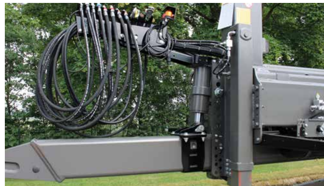
The height-adjustable towing devices are available with rubber silent blocks or with hydraulic cylinders.
