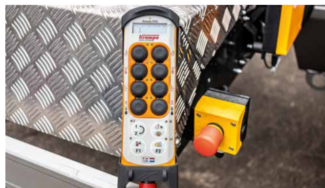
The main work cylinder, the push arm and the hydraulic container locking device can very easily be operated with the wireless remote control. Further functions are available.
